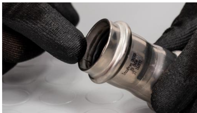
Figure 23 - Checking the sealing ring
