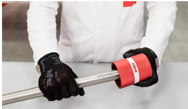
Figure 20 - Deburring the pipe
